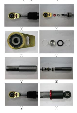
Figure 2: Components of a hybrid damper.
