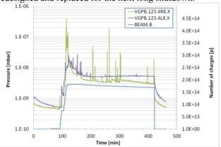
Figure 3: Pressure spikes on the vacuum RF insert modules.
