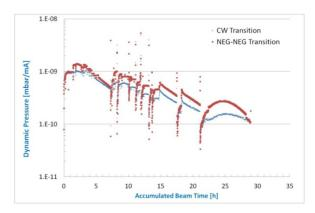
Figure 1: dynamic pressure increase in the Cold-Warm (CW) transition area and in the NEG-NEG area as a function of the beam accumulated time.
