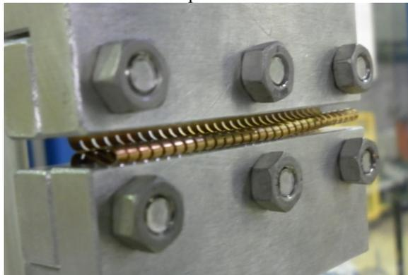
Figure 6: First fatigue tests on deformable RF fingers.
