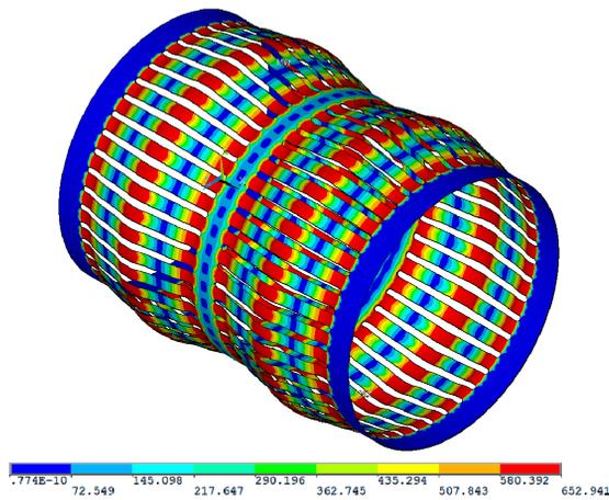
Figure 5: Von Mises stress field in extension.
