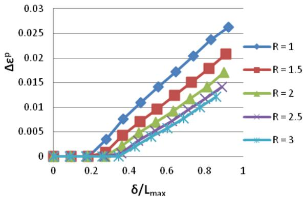
Figure 3: Influence of bending radius on the accumulated plastic strain.
