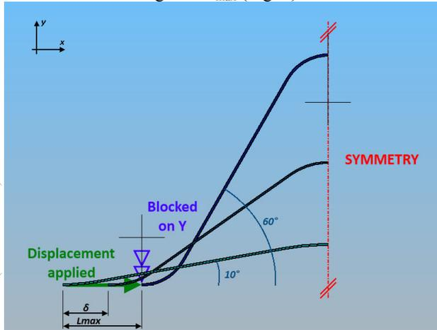
Figure 2: 2D model of a half convolution of the RF finger.
