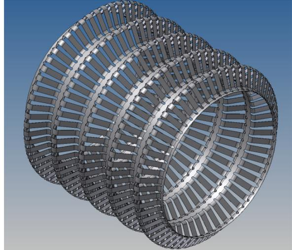
Figure 1: Deformable RF fingers in free configuration.
