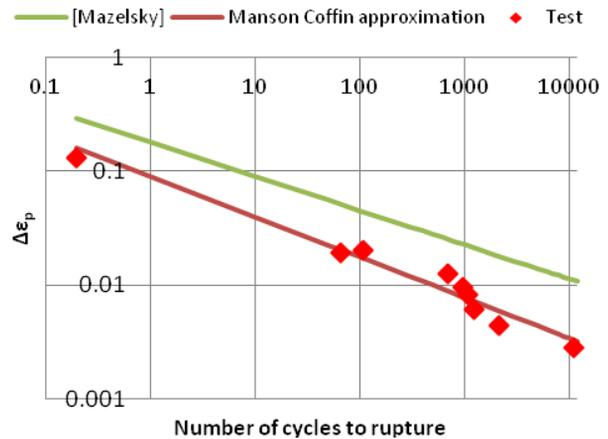
Figure 7: Fatigue curve for the deformable RF finger.
