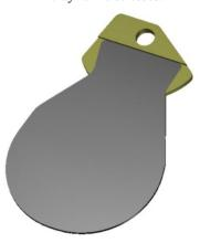
Figure 1: Dovetail connection between the glassy carbon blade and the titanium support.
