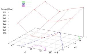
Figure 3: Influence of the dovetail geometry on stress concentration.
