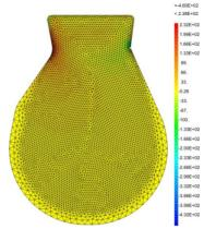
Figure 2: Principal stress field in deceleration for the dovetail geometry.
