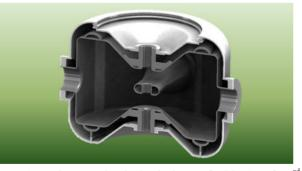
SFigure 1: The mechanical design of SSR1 of 3<sup>rd</sup> generation. A transition ring couples the niobium cavity wall to the steel vessel wall and can be seen at the bottom. The bellows is visible at the top. The niobium components are rendered in dark grey, the stainless steel ones are rendered in light grey.
