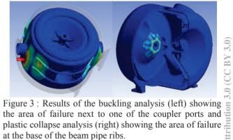
at the base of the beam pipe ribs.
