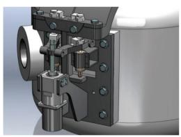
Figure 5 : The actuating elements of the tuning system.
