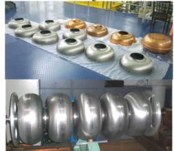
Figure 6: The pressed niobium half cells, copper half cells and EBWed cavity.
