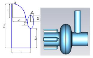
Figure 3: Cell shape and CST model of the new type single cell cavity.
