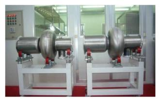
Figure 1: The deep-drawing process, the half cells and the final electron beam welded KEKB type 500MHz single cell niobium cavities in SINAP.
