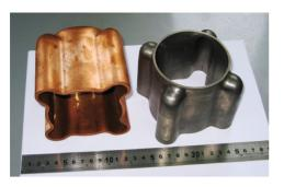
Figure 4: Scaled OFHC prototype and fabricated niobium seamless fluted beam pipe.
