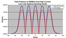
Figure 5: 500MHz 5cell cavity model by CST and field flatness output of CST and Superfish.
