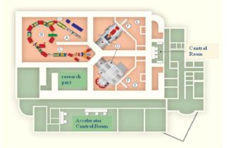
Figure 1: Proton therapy facility at PMRC. A: RFQ and DTL linac, B: proton synchrotron, C: high energy beam transport, D: rotating gantries, E: treatment rooms, F: patient beds.
