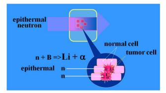
Figure 2: Principle of BNCT.
