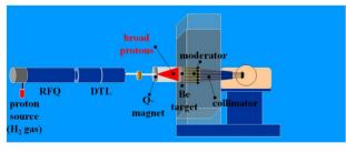
Figure 4: Layout of medical neutron accelerator at PMRC.
