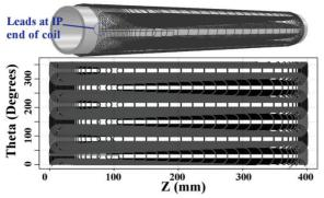
Figure 5: Example of lowest order,  $b_3$ , cancel coil pattern. The leads come out at the IP end of the magnet (same as for main coil). Non-lead end turn spacing is dramatically increased to make the sextupole gradient follow the desired cancel coil field fall-off profile.
