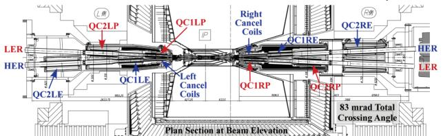
Figure 1:. SuperKEKB IR layout inside Belle-II with high energy, e<sup>-</sup>, (HER) and low energy, e<sup>+</sup>, (LER) rings indicated. #parker@bnl.gov
