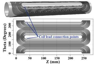
Figure 2: A planar pattern coil winding example, the single layer skew dipole pattern for QC1PL. Single layer planar coils have leads trapped at the poles.
