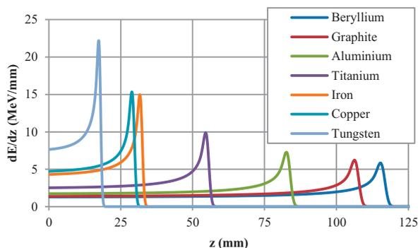
Figure 3: Energy deposition for the different materials along the axial direction.
