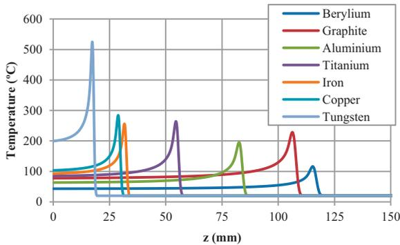
Figure 4: Peak temperature along the axial direction for each material after the first pulse.
