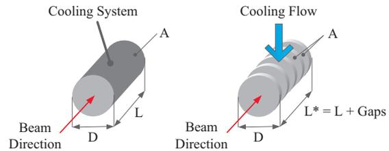
Figure 2: Geometries studied: a) Cylindrical Core (CC) and b) Circular Plates (CP).
