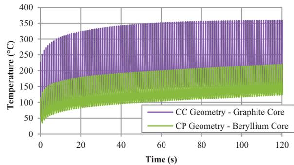
Figure 5: Peak temperature evolution in the CC geometry with graphite core and in the CP geometry with beryllium core.
