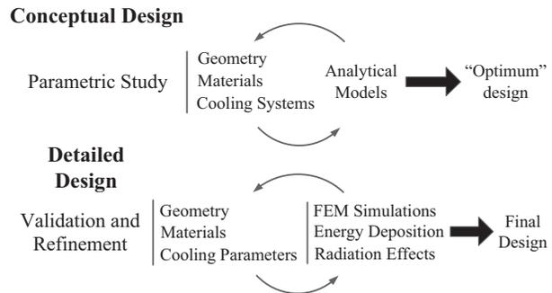
Figure 1: Diagram of the design phases for the Linac4 Main Dump.
