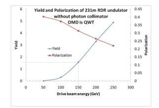
Figure 2: Yield and Polarization of RDR positron source with different drive beam energy.
