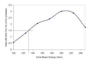
Figure 4: Yield with 60% polarization for undulator with K=0.9 and  $\lambda$ u=0.9cm.
