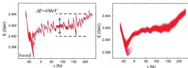
Figure 5: Longitudinal phase-space of the beam core at the exit of the spreader with laser heater off (left) and on. (IMPACT simulations.)
