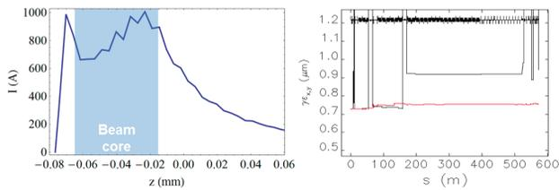
Figure 4: Beam current profile (left) and evolution of the projected transverse rms emittances along the machine.
