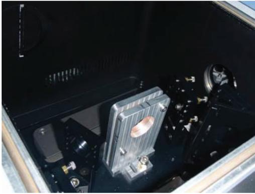
Figure 4: The removable reflectance module and home-made mirror mount.
