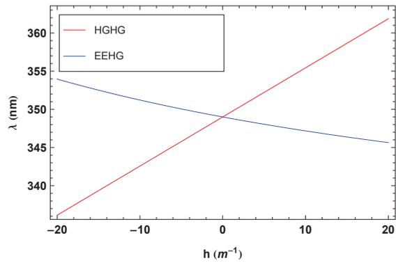
Figure 3: Central wavelength as a function of the energy chirp in the electron beam.
