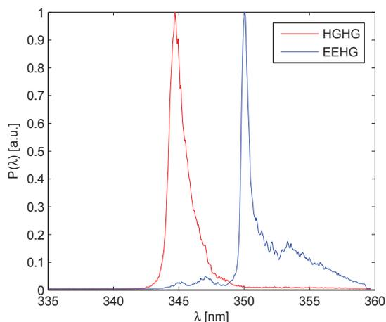
Figure 6: Measurement spectra of FEL radiation generated by HGHG and EEHG.
