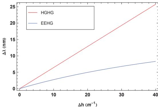
Figure 5: Spectral bandwidth increase as a function of total energy chirps in the electron beam.
