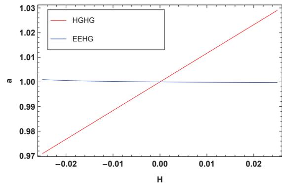
Figure 1: wavelength shift factor as a function of energy chirp in the electron beam.
