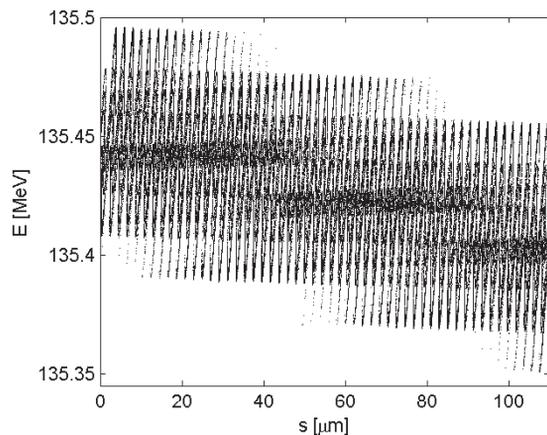
Figure 4: Phase space of the electron beam at the entrance of the radiator of EEHG.
