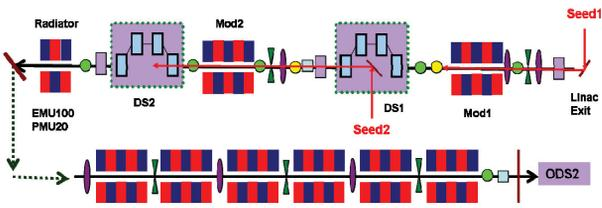
Figure 2: Layout of the experiment area of SDUV-FEL.
