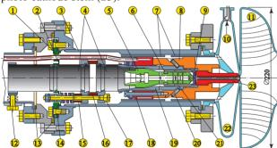
Figure 1: The sketch of the upgraded cathode insert.
