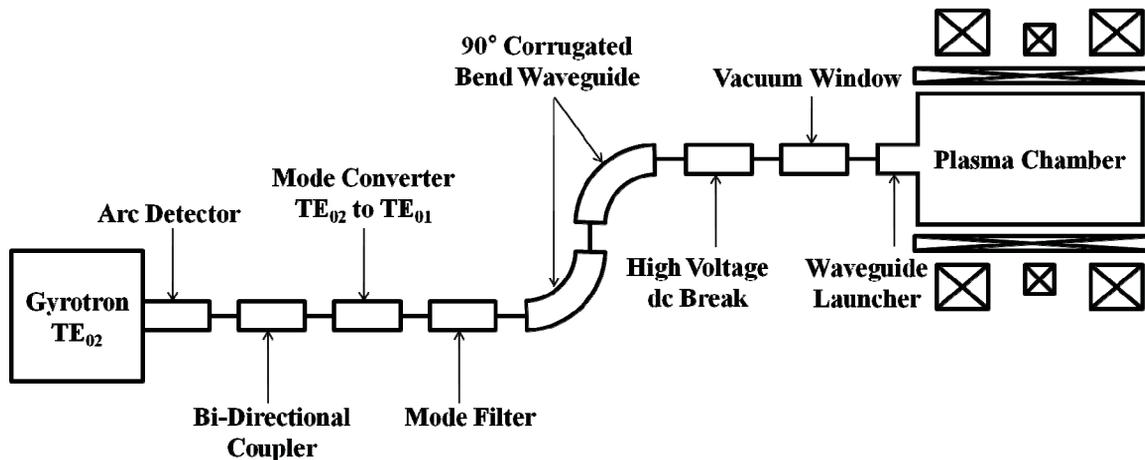
Figure 4: Schematic drawing of the 28 GHz microwave transmission line from gyrotron to ECR ion source.
