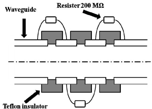
Figure 5: The design of DC break.
