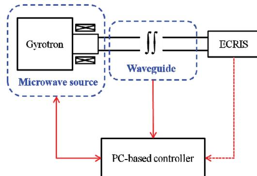
Figure 1: Diagram of microwave transmission line.
