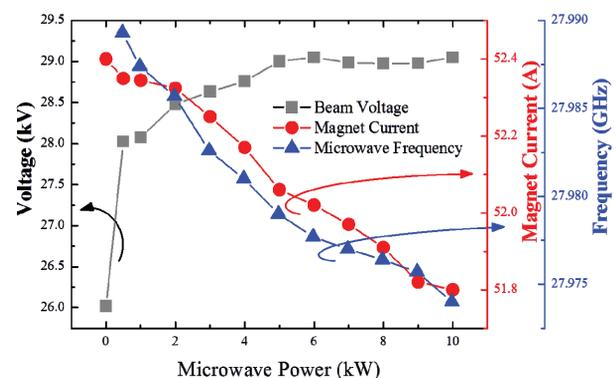
Figure 2: Beam voltage, magnet current and output frequency characteristics in gyrotron as a function of output power.
