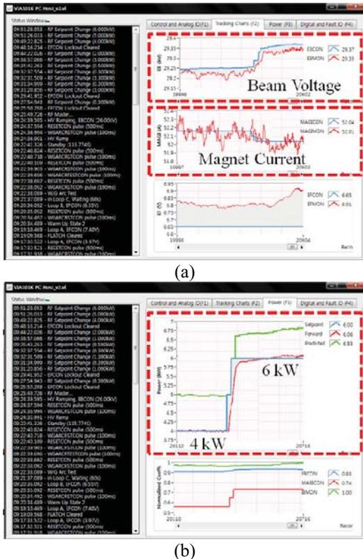
Figure 3: (a) The beam voltage and magnet current monitor of the microwave output, and (b) on screen of gyrotron controller.
