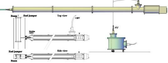
Figure 4: The Blumlein generator prototype. At the left: The Blumlein pulser as a three-coaxial line. Outer diameter of the Al tubing is 7", length of each section ~1.5 m. In the final model diameter will be reduced to 4" OD. Inner volume filled with oil. T stands for the thyratron.
