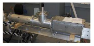
Figure 5: The thyratron housing with HV input.
