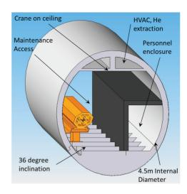
Figure 5: Cross-section of the decay ring tunnel showing the stepped floor and personnel enclosure.
