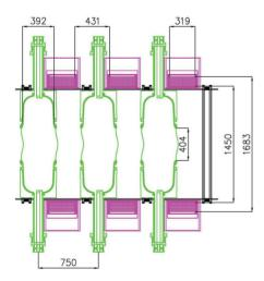
Figure 3: Schematic drawing of the buncher module showing the arrangement of the coils, cavities and RF power input couplers.
