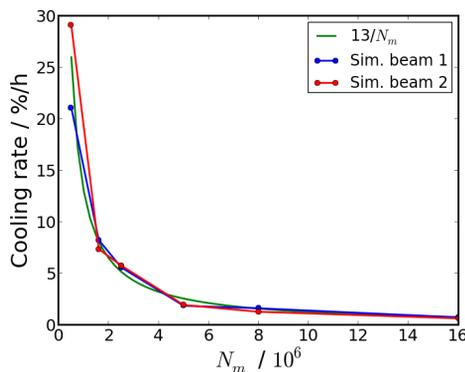
Figure 4: Cooling rate as a function of the number of macro particles and a hyperbola.
