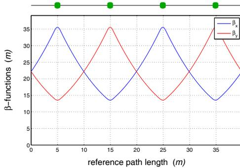
Figure 2: Betatron functions along two  $54^\circ$  FODO cells.
