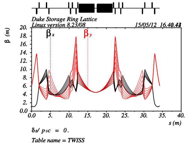
Figure 1: SSS Lattices of different OK-5 wiggler strength for two OK-5 wigglers configuration. The energy normalized wiggler strength  $k$  varies from  $0 \text{ GeV}^{-2}$  to  $0.7 \text{ GeV}^{-2}$ . Black lines represent  $\beta_x$ , and red lines represent  $\beta_y$ .
