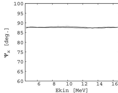
Figure 3: Horizontal local phase advances versus kinetic energy in the Straight FFAF line with TOSCA map (plain) and with measured map (dotted).
