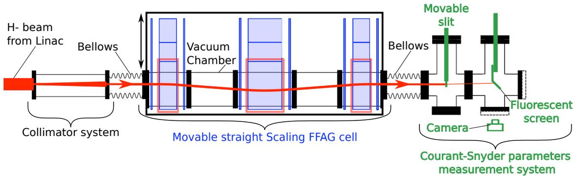
Figure 1: Schematic view of the Straight Experiment.
