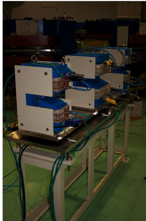
Figure 6: Picture of the straight scaling FFAG magnets prototype.
