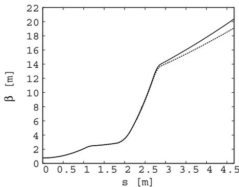
Figure 5: Horizontal betafunctions in the Straight FFAG line with TOSCA map (plain) and with measured map (dotted).
