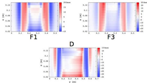
Figure 2: Difference of the vertical magnetic field in the mid-plane in Gauss between the TOSCA field map and measured field map of the magnets F1 (top left), F3 (top right) and D (bottom).
