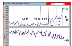
Figure 4: Beam dimension (in  $\mu$ m) at the SLM turning off, progressively, all electrodes.
