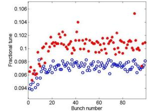
Figure 3: horizontal fractional tune as a function of bunch number (blue curve: electrodes ON,  $I_B$ =550mA; red curve: electrodes OFF,  $I_B$ =600mA).
