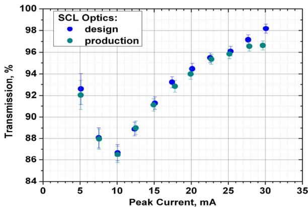
Figure 2: The proton beam transmission in the linac.
