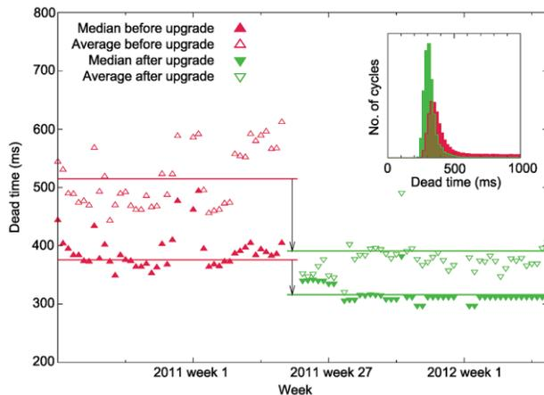
Figure 3: Dead time between cycles in therapy mode (weekly analysis)
