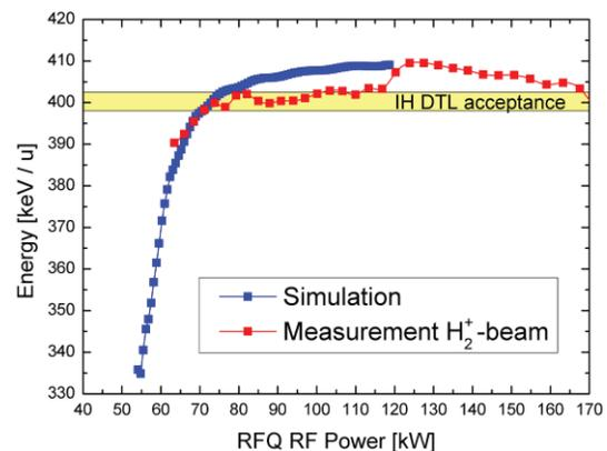
Figure 2: Measurement of the RFQ output energy in comparison to the simulation for a  $\text{H}_2^+$  beam
