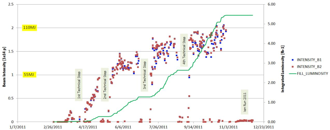
Figure 2: Increase of beam intensities and integrated luminosity during LHC operation 2011.
