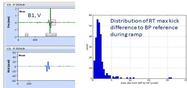
Figure 5: Orbit bump  $>2\text{mm}$  developing during a ramp of fill 1717. The system clearly identifies the unusually high kick applied by calculating the difference between the applied kick and the BP reference.
