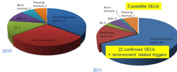
Figure 4: Fraction of false dump triggers from machine protection systems in 2010 (left) and 2011 (right).
