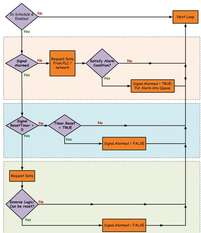
Figure 2: Architecture of the decision loop of the alarm system
