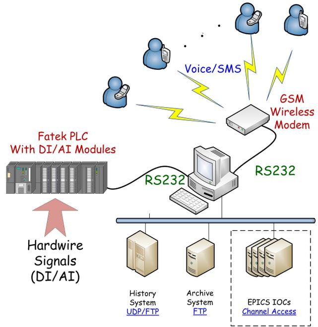
Figure 1: Hardware structure of the broadcasting system
