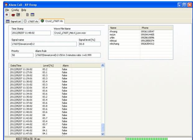
Figure 5: Screenshot of the alarm broadcasting software
