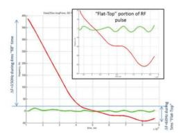
Figure 2: Detuning of the cavity ( $Q_L$ =3\*10<sup>6</sup> and Eacc=18MV/m) by Lorentz forces during a 9ms pulse. Red curve is cavity's LFD when piezo compensation is OFF. Green curve is the cavity's detuning when cavity resonance control with piezo tuner and adaptive compensation algorithm is active. Insert: zoomed window shows LFD detuning during 5ms "Flat-Top" portion of RF pulse (red-piezo OFF; green-piezo ON).
