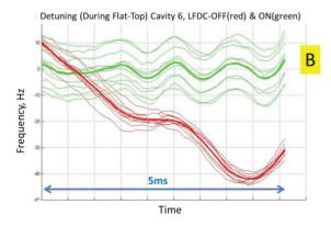
Figure 5: (A): Pulse-to-Pulse Detuning Variation (RMS Detuning) for E<sub>acc</sub>=10;15;20MV/m. (B): Detuning (during 5ms Flat-Top) for the 10 RF pulses with LFDC system ON (green) and OFF (red). Thick line is average of 10 pulses.
