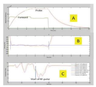
Figure 1: LFD Compensation in C5 and C6 during a 9ms RF pulse at  $E_{acc}$ =25MV/m and  $Q_L$  = 6\*10<sup>6</sup>. (A): Baseband envelopes of the forward and cavity field probe signals. (B): Residual detuning using following compensation. Adaptive LFD algorithm. (C): Piezo drive waveforms.
