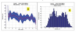
Figure 3: Residual Detuning over 30 minutes during operation at  $Q_L$ = $10^7$  and  $E_{acc}$ =24.5 MV/m. (A) shows the detuning waveforms of 1800 pulses collected over a 30 minute period while (B) shows a histogram of the average detuning for the same sample.
