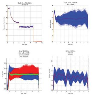
Figure 4. Top Plots: Forward Power and Phase signals of C5 and (bottom plots): Amplitude (C5, C6, Vector sum) and Phase Stability (Vector Sum) over 30 minutes during operation at  $Q_L$ =10<sup>7</sup> and  $E_{acc}$ =24.5 MV/m.
