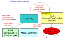
Figure 4: Local and global compensation schema for insertion device.
