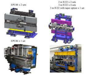
Figure 1: Insertion devices of TPS in the phase-I.
