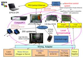
Figure 2: Basic hardware configuration for TPS insertion devices in Phase-I.
