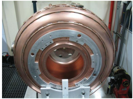
Figure 8: The first MICE cavity electro-polished at LBNL in May 2012.
