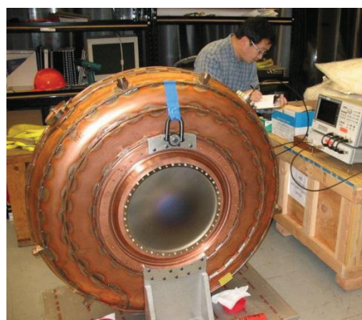
Figure 5: MICE RF cavity measurements with curved beryllium windows at LBNL.
