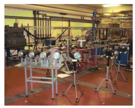
Figure 4: The  $^8B$  experiment. 8 Photo Multiplier Tubes cover neutron angles from  $15\,^\circ$  to  $140\,^\circ$  in the lab frame.
