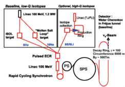
Figure 1: The CERN Beta Beam. The beta active isotopes are accelerated to the Decay Ring: <sup>6</sup>He/<sup>18</sup>Ne (low-Q) with a detector in Fréjus (baseline) and optionally <sup>8</sup>Li/<sup>8</sup>B (high-Q) with a detector at 700 km (Gran Sasso or Canfranc).
