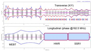
Figure 4: Transverse (mm) and longitudinal (degrees of 162.5 MHz) rms beam envelopes from the RFQ exit (2.1 MeV) to the exit of the SSR1 cryomodule (22 MeV). Peak beam current is 5 mA  $(1.9 \times 10^8 \text{ ppb})$ .
