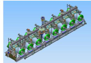
SFigure 5: The HWR cavity and solenoid string assembly.
