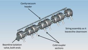
Figure 6: The SSR1 cavity and solenoid string assembly.
