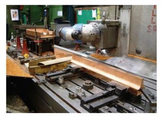
Figure 1: RFQ major and minor vanes being machined.
