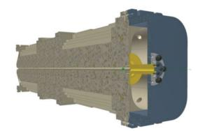
Figure 4: Section view of bead-pull / RF test end flange.
