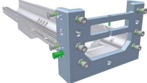
Figure 2: Jig used for RFQ vane to vane alignment.
