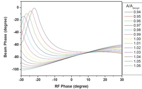
Figure 3: Beam phase as a function of RF phase for DTL101.
