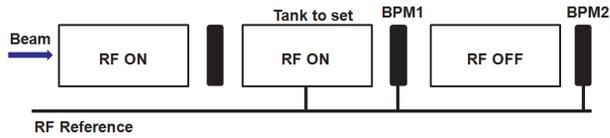
Figure 2: Schematic plot for beam phase measurement of a DTL tank.
