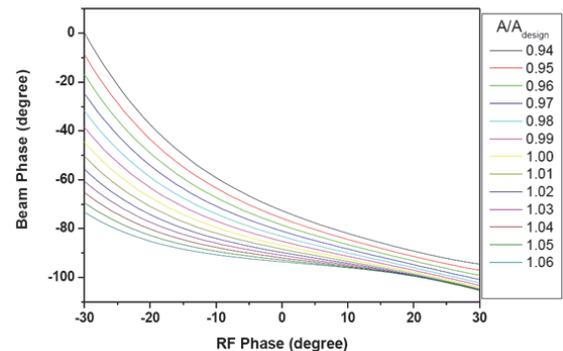
Figure 5: Beam phase as a function of RF phase for DTL102.
