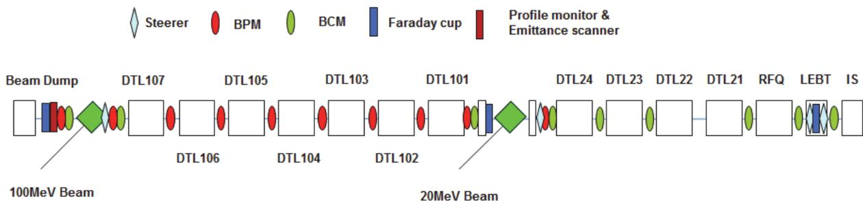
Figure 1: Layout of beam diagnostics in PEFP linac.
