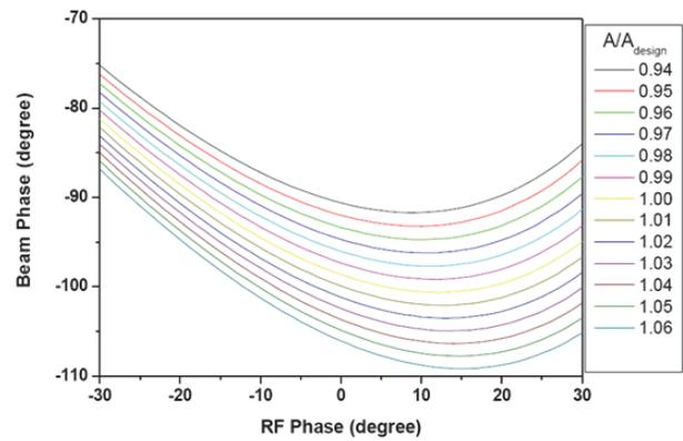
Figure 10: Beam phase as a function of RF phase for DTL107.
