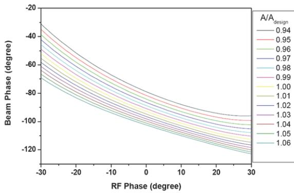
Figure 5: Beam phase as a function of RF phase for DTL103.
