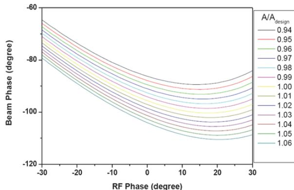
Figure 9: Beam phase as a function of RF phase for DTL106.
