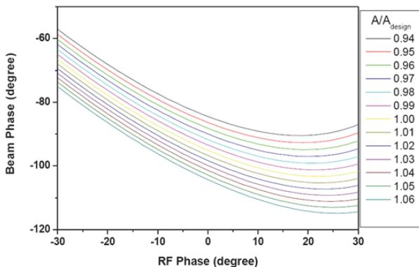
Figure 8: Beam phase as a function of RF phase for DTL105.
