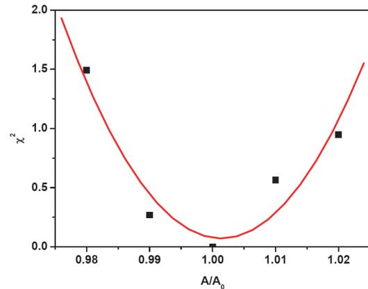
Figure 4: Amplitude determination by comparing the simulation results with the artificial experimental result for the relative amplitude of 1.0.
