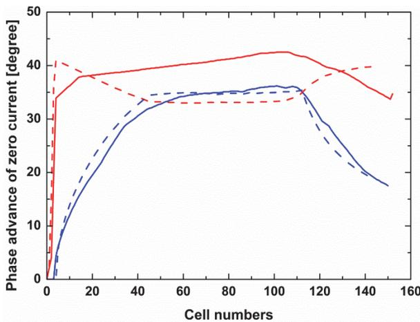
Figure 1: Comparison of the phase advance of zero current in the transverse (red) and longitudinal (blue) plane for both the traditional design (dash line) and optimized one (solid line).
