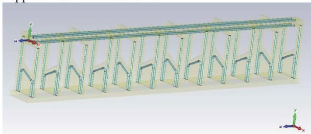
Figure 5: Cooling channel in the structure.
