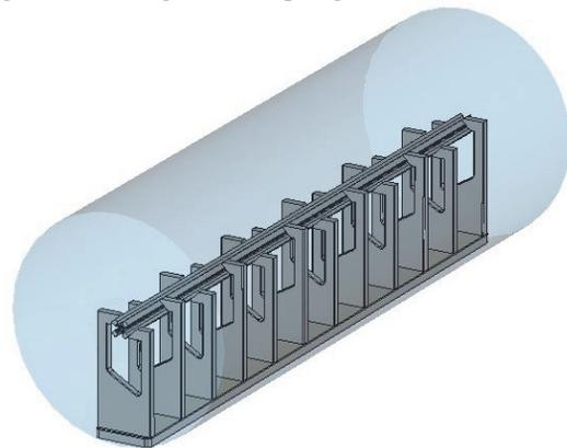
Figure 3: Resonance structure of SSC-LINAC RFQ.
