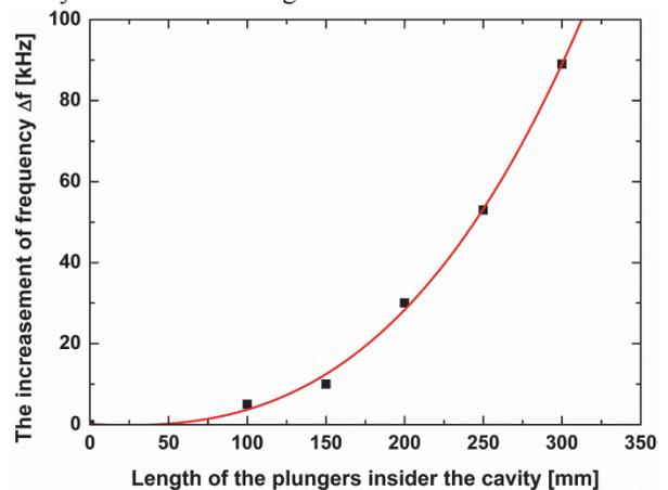
Figure 7: The change of frequency caused by all four plungers.
