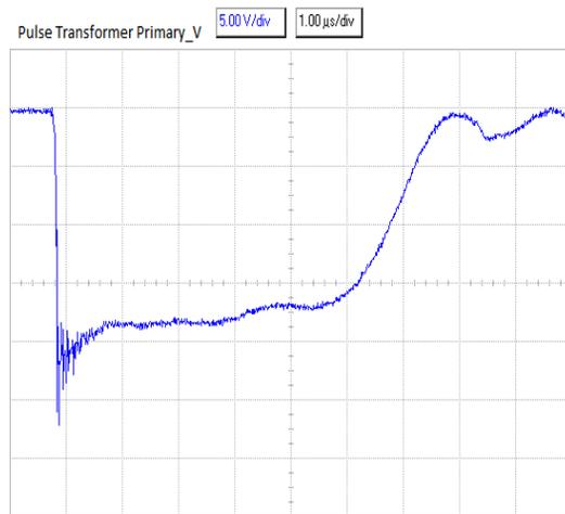
Figure 5: Test results at ANL using S56-12 showing primary pulse transformer voltage at a 1000:1 calibration.
