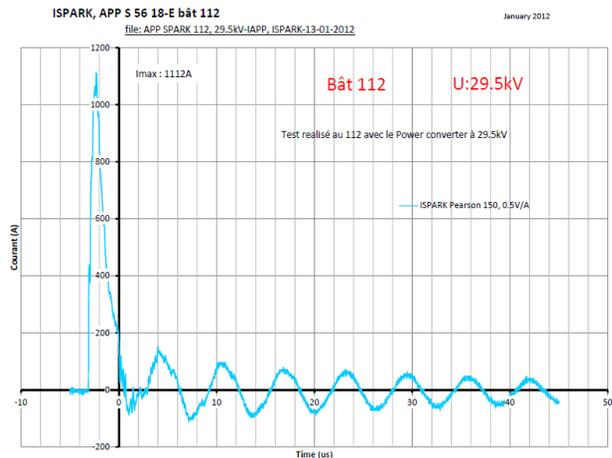
Figure 8: Crowbar operation of a S56-18 at CERN.
