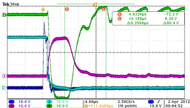
Figure 7: S60-2-16 solid state switch test results from SLAC showing pulse voltage and current. Ch1--Modulator trigger in; Ch2--PFN charging voltage (1000:1); Ch3--Switch current (180:1); Ch4--Klystron beam voltage (4860:1).
