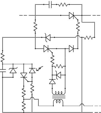
Figure 2: Self-powered trigger circuit.
