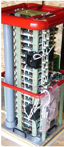
Figure 6: S60-2-16 solid state switch at SLAC.
