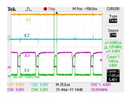
Figure 5: The PWM waveform of one arm regulation.
