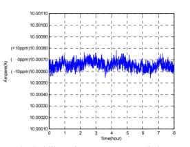
Figure 9: Stability of output current of the corrector magnet power converter within 8 hours.
