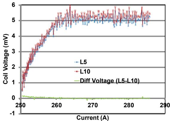
Figure 9: There is no noticeable voltage difference between coil#5 and #10 at 4.2K.
