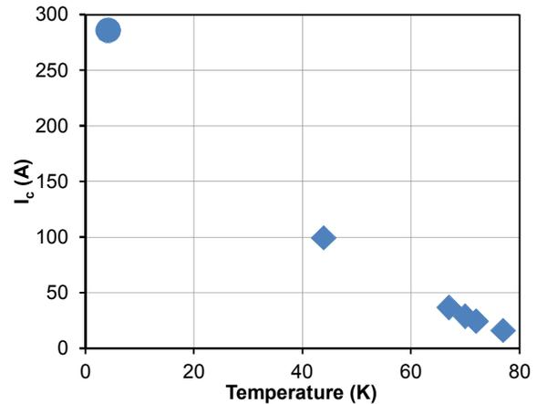
Figure 10: The critical current is plotted as a function of temperature. Although critical current is only 16A at 77K, it could be above 285A at 4.2K (shown as a circle).
