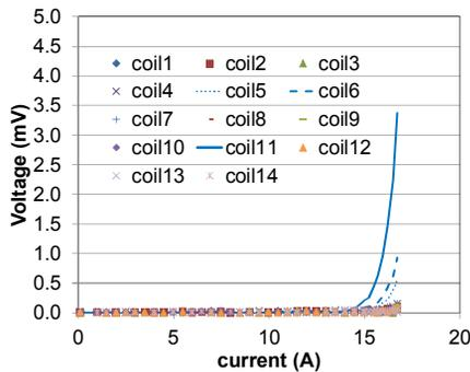
Figure 4: Measured voltage at 77 K across each of 14 coils when powered in series. Coil #11 becomes resistive first followed by #6 and #5.
