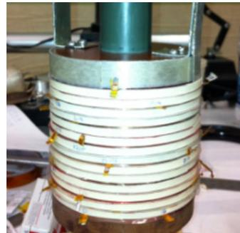
Figure 2: Photograph of the insert solenoid.
