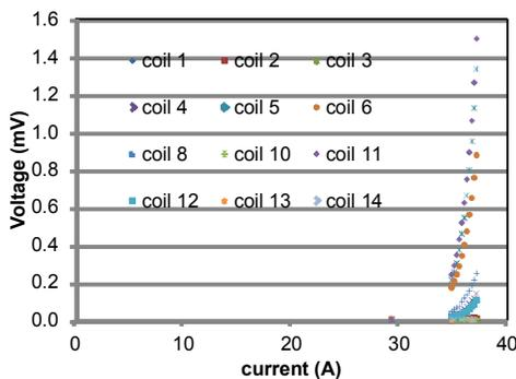
Figure 5: Coil #11 and #5 became resistive first followed by #6 at 67 K.
