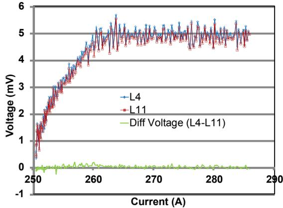
Figure 8: There is no noticeable voltage difference between the pairs #4 and #11 at 4.2K.
