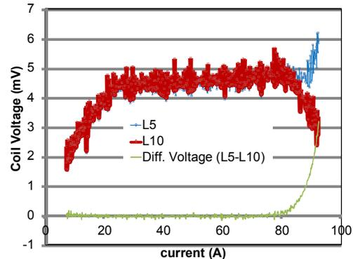
Figure 6: Coil #5 became resistive and voltage difference between #5 and #10 exceeded 2mV, so the power supply shut down at 92 A at 44 K.
