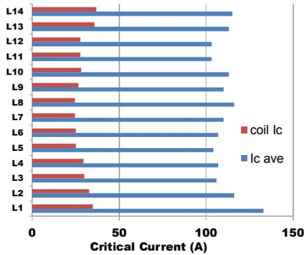
Figure 3: Critical current of 14 coils (measured at BNL) and critical current of conductor (measured at SuperPower) at 77 K used in the solenoid.
