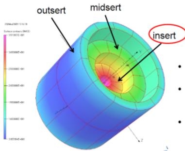
Figure 1: PBL High field solenoid consists of three solenoids. The insert and the midsert will be made with 2G HTS and outsert with LTS.
