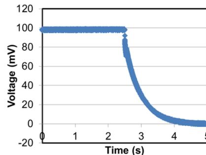
Figure 7: The coil current after the power supply shut off is plotted as a function of time.
