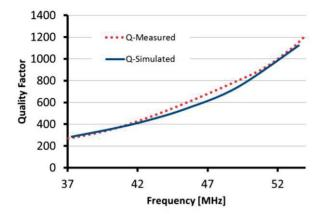
Figure 5: Simulated quality factor versus frequency of the Booster cavity compared to measured curve.
