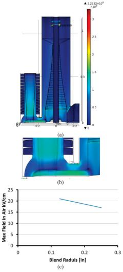
Figure 4: Simulated electric field (55 kV gap voltage): (a) on the surface of the Booster cavity (b) on the tuner connection, (c) maximum electric field in air versus edge blend radius.
