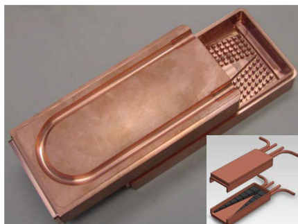
Figure 2: Prototype HOM damper with copper pinbed substrate. Inset shows LOM damper with SiC tiles.
