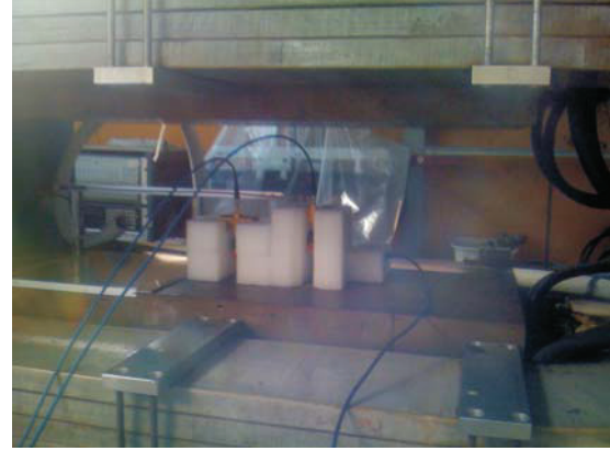
Figure 4: Aperture of the biasing magnet with sample holders and Hall-probe.
