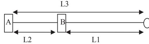
Figure 1: Layout of quads and flags for resolution measurement.
