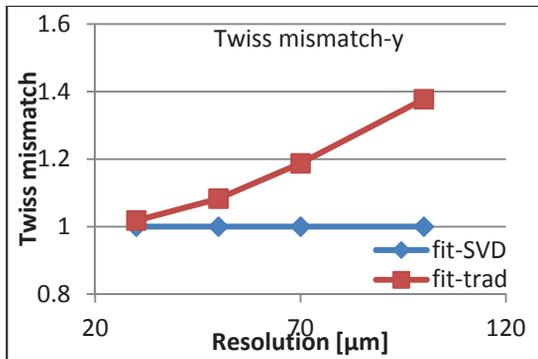
Figure 3: The fitted Twiss mismatch parameter vs. input flag resolution in x and y plane.
