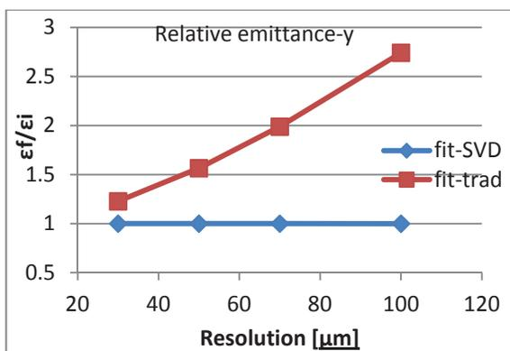
Figure 4: The fitted relative emittance vs. input flag resolution in x and y planes.
