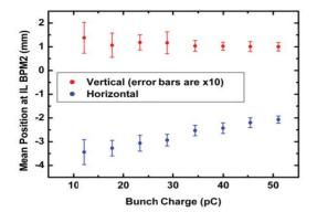
Fig. 1: Bunch offset vs charge.
