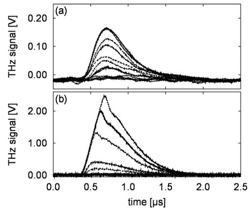
Figure 6: Oscilloscope traces of laser-induced THz signals with moderate amplitude (a). The different traces were recorded by reducing the spatial overlap between laser pulses and electron bunch. At THz signals with higher amplitude, a saturation effect in terms of a constant rising edge steepness is visible (b).
