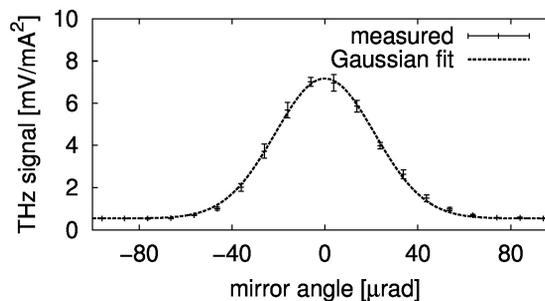
Figure 3: THz signal versus horizontal angle of a mirror in the laser beamline (BL3). The square root of the THz signal is proportional to the convolution of the horizontal electron bunch and laser pulse profiles.
