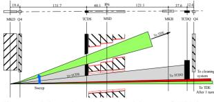
Figure 1: Schematic and functional layout of TCDS and TCDQ diluter elements.
