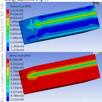
Figure 5: YY stress field (kPa) at  $t = 19.5 \ \mu s$  (top) and at the end of the energy deposition (bottom).
