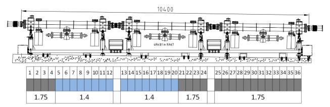
Figure 2: Proposed layout of a 3-tank TCDQ system (above), with a total length of 10.4 m, installed on a mobile support girder to allow precise positioning of the absorber blocks with respect to the beam position. Below a schematic representation of the 36 absorber blocks inside the tanks with densities of 1.75 or  $1.4 \text{ g/cm}^3$ .
