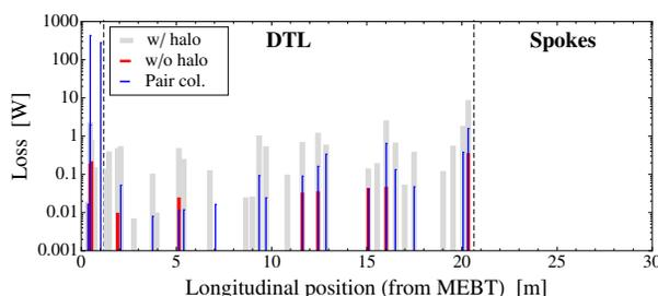
Figure 6: Beam losses for the *90° Pair Scheme*. The collimators must absorb as much as a few hundred Watt to reduce the losses to the level of the no halo case.
