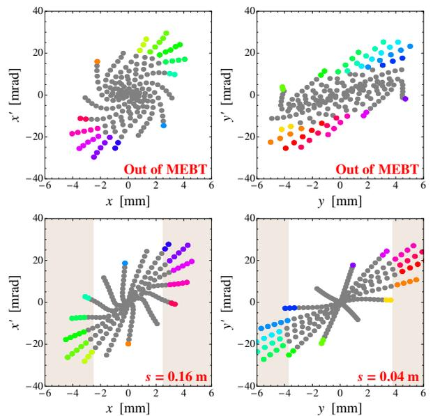
Figure 5: Sample particles ending up beyond  $5\sigma$  at the end of the MEBT (top) and their phase space positions at the proposed collimator locations for the *Single Scheme* (bottom). Brown parts represent the collimator plates.
