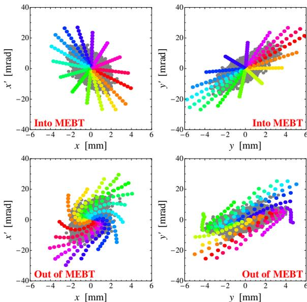
Figure 3: Particle distributions in the phase space going into the MEBT (top) and out of the MEBT (bottom). The gray parts represent the beam core.
