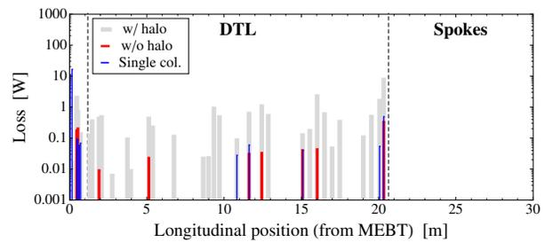
Figure 7: Beam losses for the *Single Scheme*. Each collimator only needs to absorb 10 W unlike the case of the *90° Pair Scheme*.
