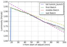
Figure 3: Bunch-by-bunch luminosity averaged over each of the three batches.
