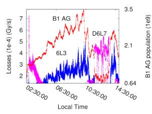
Figure 6: B1 AG population (red), losses at betatron collimator TCP.D6L7.B1 (magenta) and momentum collimator TCP.6L3.B1 (blue).
