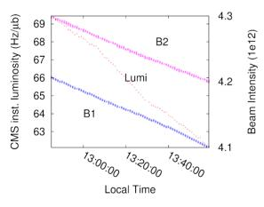
Figure 2: Luminosity vs. time (red) shows a kink at about 13h10 corresponding to the moment B1 and B2 cleaning is switched on. The second kink at about 13h34 corresponds to the moment the cleaning is turned off. The BCT (blue for B1, magenta for B2) does not show kinks.
