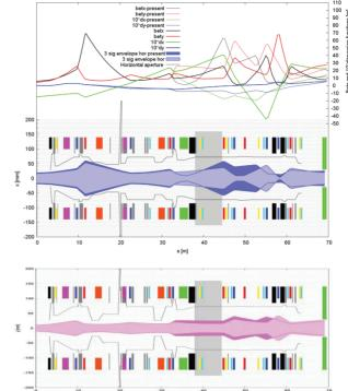
Figure 5: Optics matched to foreseen upgrade optics for HI beams with only local perturbation at PS injection.
