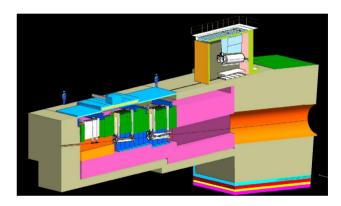
Figure 2: Section of the Target Hall complex and the Decay Pipe.
