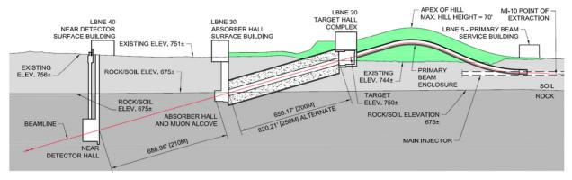
Figure 1: Longitudinal section of the LBNE Beamline facility in the MI-10, Shallow beamline configuration.
