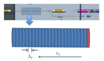
Figure 1: Top: Lay out of CEC PoP experiement. Bottom: Cartoon for layout of electron beam slices. Red slice corresponds to the one with initial non zero bunching factor; blue slices corresponds to the zero bunching factor generated by 'quiet start algorithm' in Genesis. Each slices has the length of the resonance radiation wavelength.
