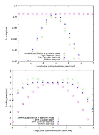
Figure 4: The output bunch factor (top) and phase (bottom) that the ion encounters at the exit. The bunch length is rms value.
