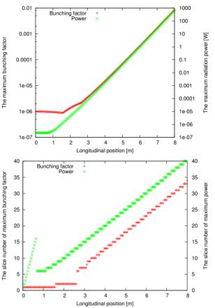
Figure 3: The maximum radiation power and bunching factor values (top) and their longitudinal positions with the unit of  $\lambda_r$  (bottom) along the FEL process.
