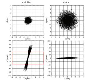
Figure 3: Initial (left) and final (right) transversal beam profile and beam emittance. The initial energy spread of the beam was  $\pm$  6.1 %. Particles within a cone of  $\pm$  37 mrad have been accepted by the beamline.
