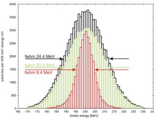
Figure 4: Histograms of the energy distribution of the particle bunch calculated for 100000 particles at different positions. At the start of the bunch the energy spectrum had a width of ±24.4 MeV (black graph). After collimation due to the geometric acceptance of the transport channel the width is reduced to ±23.4 MeV (green graph). After further collimation at the aperture the energy spread is reduced to  $\pm 9.4$  MeV (red graph).
