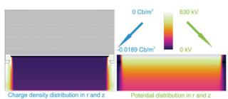
Figure 1: Results of self consistent simulation of GL2 shown in false colour representation. The left hand plot shows the configuration with coil and electrodes together with the electron charge density, the right hand plot shows the potential distribution of the lens in equilibrium.
