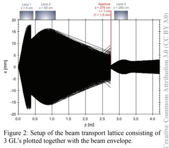
Figure 2: Setup of the beam transport lattice consisting of 3 GL's plotted together with the beam envelope.
